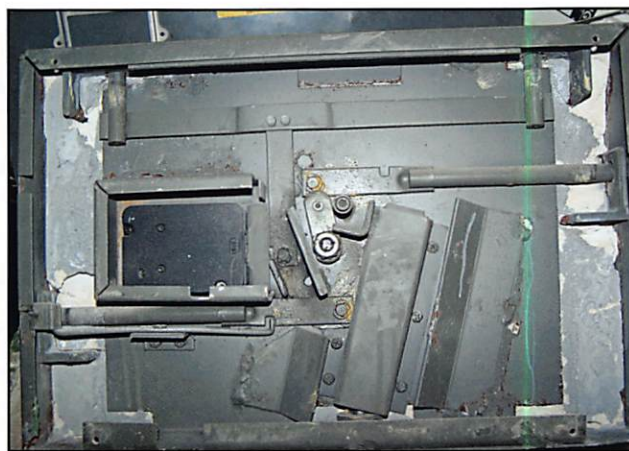
Photo 4 shows the back of the drawer head. The back cover plates for the lock were missing. Since the container would not meet specification without them, removal from service would have occurred even if the container had been repairable.
