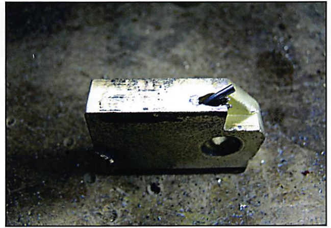
Photo 8 show the lock bolt with the magnetic pin sticking out of the side of the bolt.
